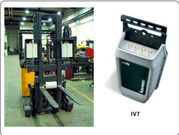
**Figure 7: Forklift Mounted Interrogators**
