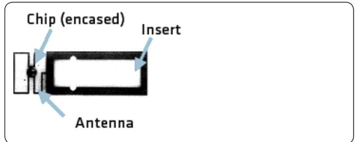
**Figure 2: Inlay–RFID Tag Components**
