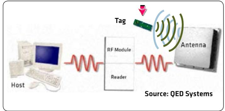
**Figure 1: RFID System Components**
