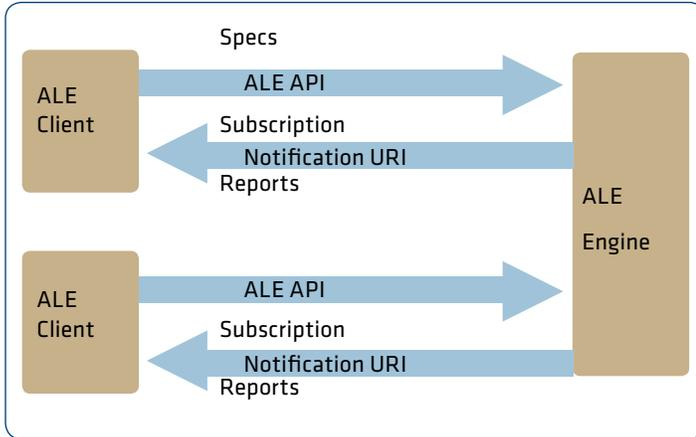
The ALE interfaces are based on XML. An ALE engine is configured using XML documents called specs (e.g., ECSpec, CCSpec, ...). Specs are communicated from an ALE client to an ALE engine via a web services interface called the ALE API (WS-i compliant). An ALE engine communicates its reports as XML documents. These reports can be communicated via files, HTTP, or other vendor-specific mechanisms such as message-oriented middleware (e.g., MQ Series).
