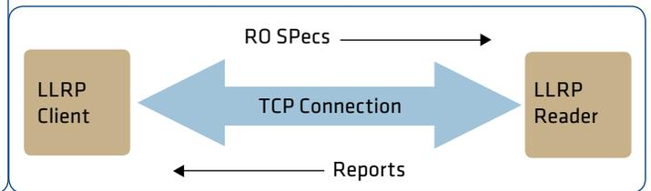
LLRP restricts readers to accepting a single TCP connection. This one connection is used to send commands from the client to the reader and for the reader to return command responses and to send reports back to the client. In addition to sending reader operation specifications (RO Specs) to the reader, an LLRP client
