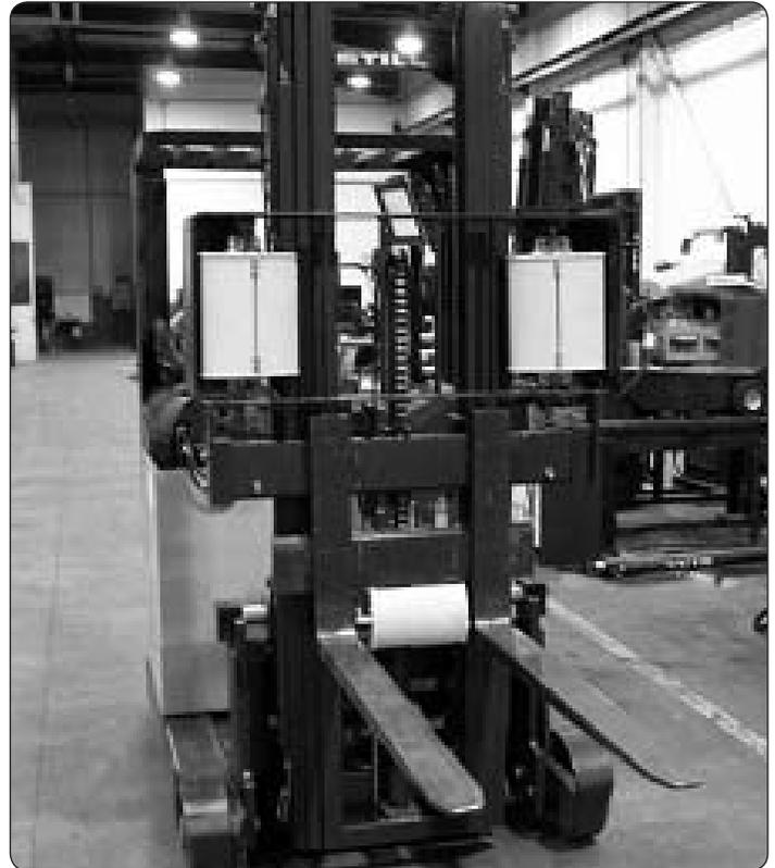
Figure 7: Forklift Mounted Interrogators
